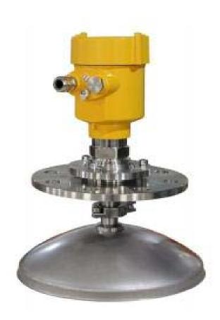
26G HF radar level measuring instrument, measuring the maximum distance up to 80 meters. The antenna is further optimized; new fast microprocessor can perform higher-rate signal analysis and processing, so that the meter can be used in reactors, solid silos, etc.
