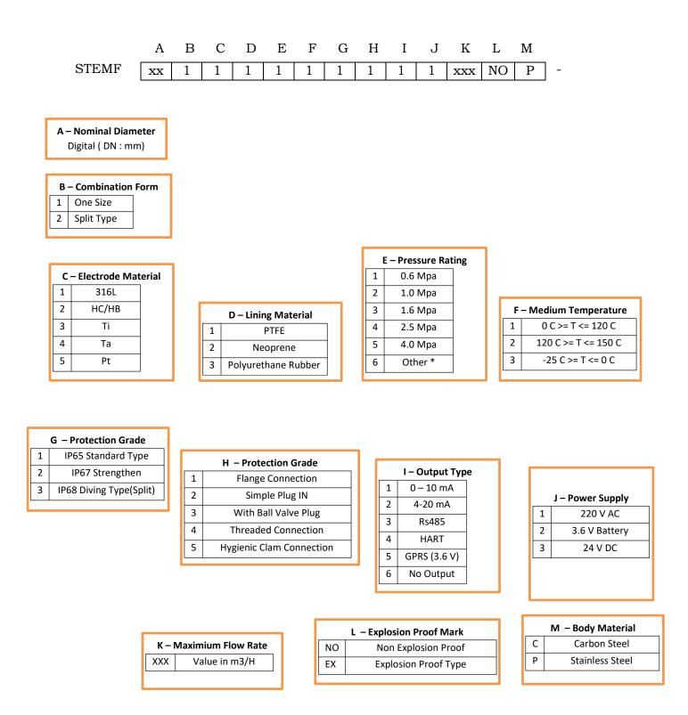
You can according to the table to choose corresponding flow electromagnetic flow meter, If the choice of electromagnetic flow meter and the inner diameter of the pipe diameter does not match the process, Should be the pipe or tube expanding.
